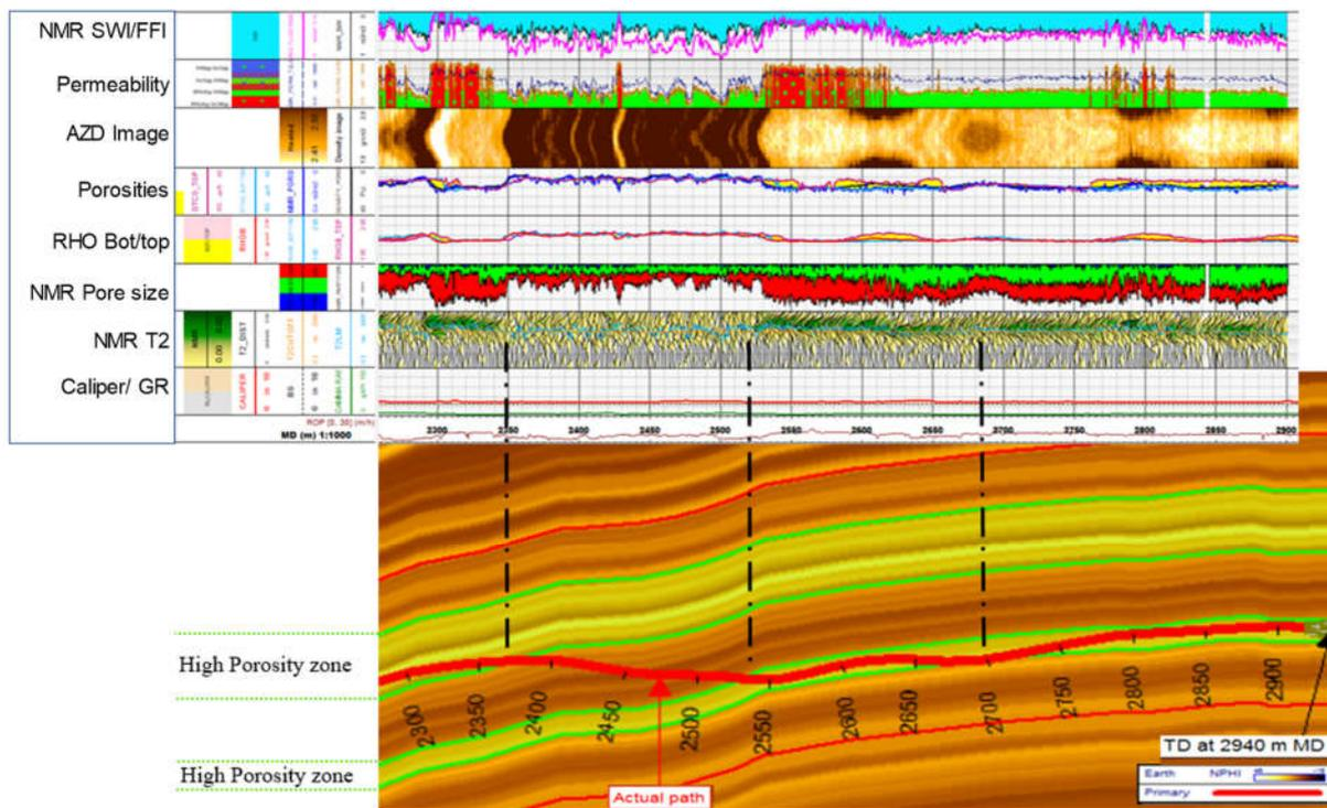
**Figure 2** The analysis of NMR logs together with sonic and density images allows for a quick evaluation of reservoirs quality and rock permeability distribution to highlight intervals with higher flow rate potential.
