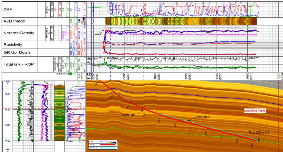
**Figure 1** Geosteering window: top, real-time parameters from mud logging (geochemical), LWD and drilling parameters; bottom left, logs from vertical offset wells; bottom right, curtain section with the planned and actual well trajectory plotted against a layered reservoir model
