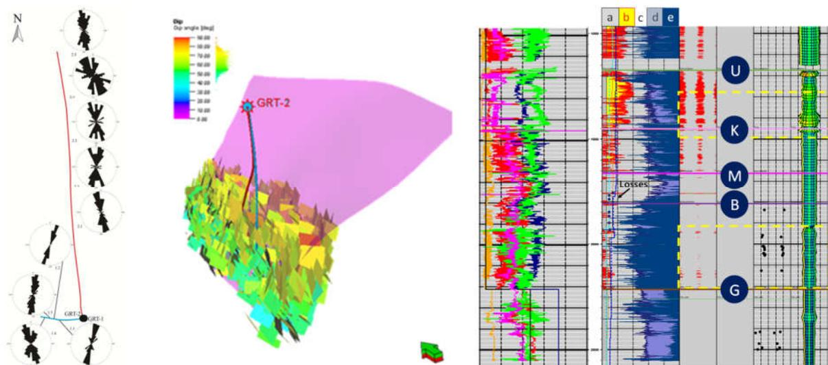
*Left: rose diagrams representing natural fracture strikes along the GRT-1 and GRT-2 trajectories and reconstructed natural fracture network model.*
