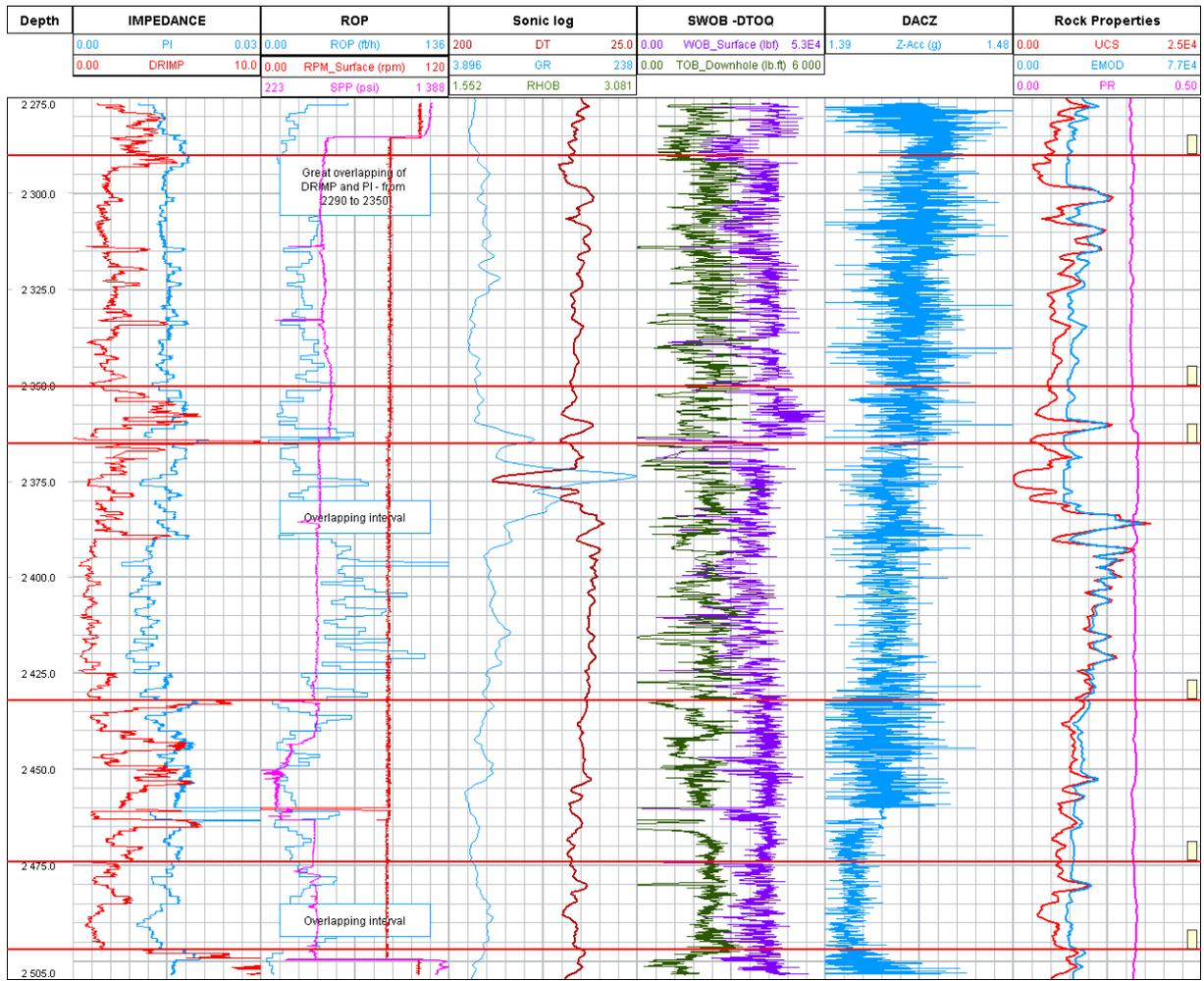
**Using the Bit to measure How Rock Reacts to Force: An In Situ Rock Mechanical Measurement,**
